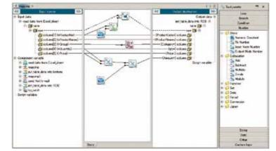
Mapper is a function that converts input/output data. It not only associates input items with output items, but also achieves flexible conversions by being able to combine over 140 functions such as calculations, string processing, condition judgment and date processing.
