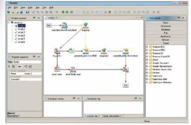
Designer is a tool to create a data integration script. Numerous functions are available such as data input/output, branching, looping, and setup of variables and conversion. Drag and drop icons to a canvas can create the flow of processing just like a flowchart.
